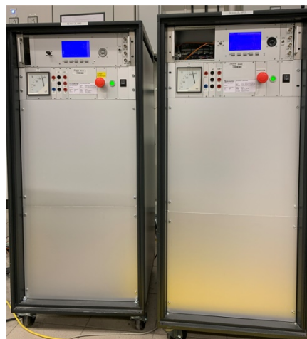
Figure 6: Inverter (left) and converter (right).
