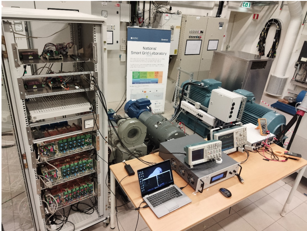
Figure 6: Experimental setup of three three-level inverter fed two OEWIM drive
