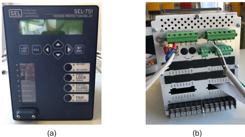
Figure 10: Protective relay used for the test, (a) front plane, (b) back plane showing direct connection of voltage and current signals.
