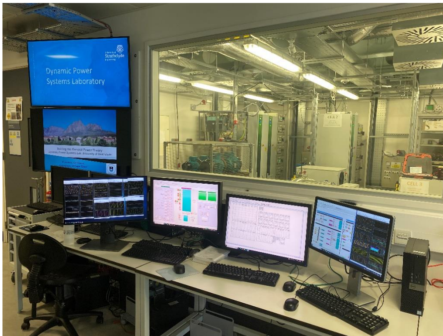
Figure 11: Photo of control room with multiple screens to monitor parameters and measured quantities in the 10 kW converter controller, RSCAD simulation model, the dc-power source and 90 kVA power amplifier. The 10 kW converter and 90 kVA power amplifier can also be observed in the experimental testing room.
