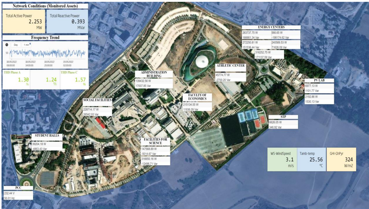
Figure 18. Real-time simulation environment UCY campus microgrid model integrated with voltage state estimator.
