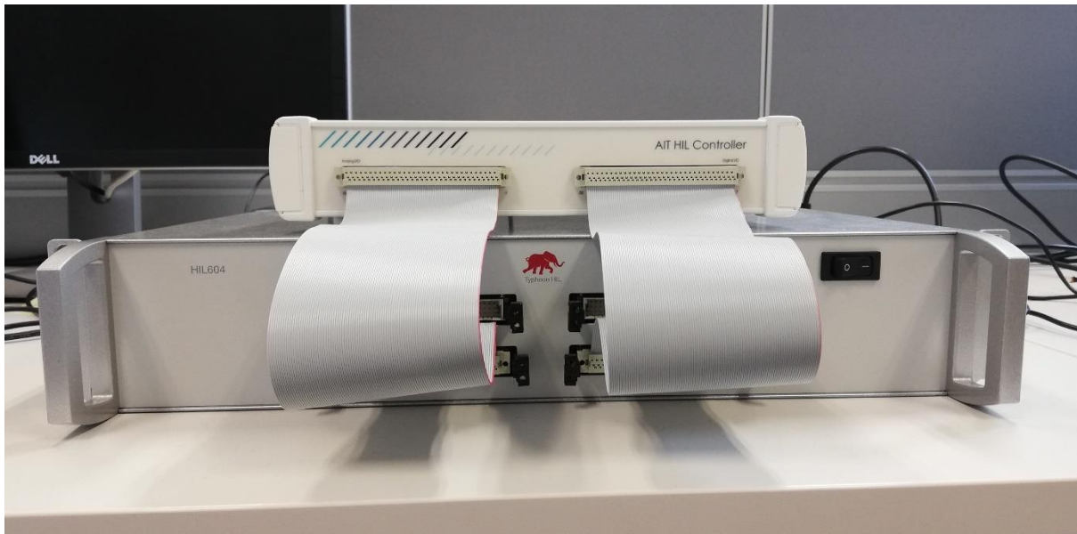
Figure 3. Typhoon HIL real-time simulation test-bed with AIT HIL controller at AIT.
