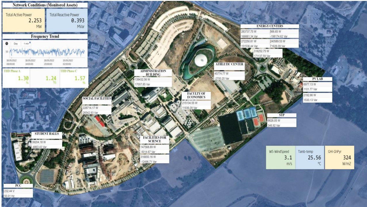
Figure 20. UCY microgrid real-time simulation platform dashboard.
